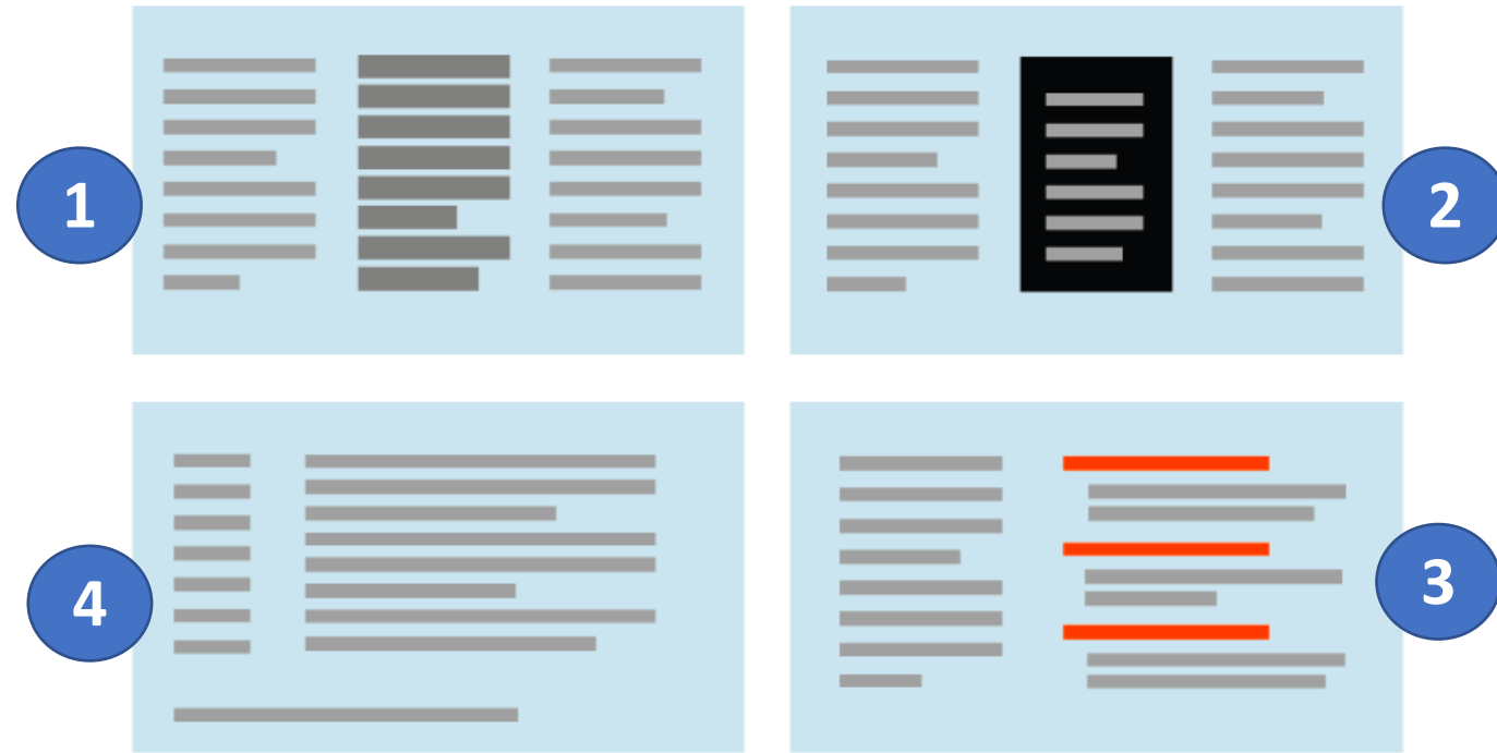
Figure 4-2. Ways to emphasize blocks of text or small items (clockwise from upper left): density, background color, rhythm, and position and size
